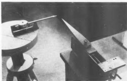
FIG. 2. Set-up of radium capsule and condenser ionometer.
